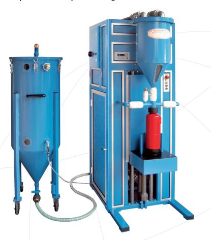
The unit operates within the filling tolerance indicated in the EN3 standards. Adjustment of the value of the filling weight has to be effected at the scale display; adjustment of the filling parameters depending on extinguisher type are effected by the text display. Height adjustment of the weighing platform takes place by screw-drive.
