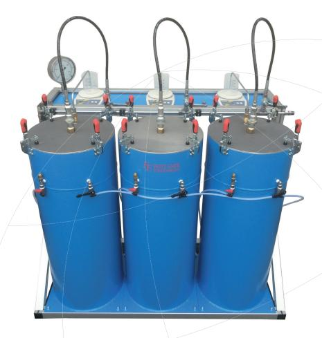
The mobile Hydrotest Unit HD-CFK-3 with three test benches is used for simultaneous pressure testing of three cylinders made of composite materials, steel or aluminum with a water volume up to 18 liters and a test pressure of 450 bar. The pressure test procedure is carried out in the volumetric expansion method (Water Jacket). In this case, the volumetric expansion of the cylinder to be tested is measured and the expansion in the measuring cup is collected and displayed on a Balance.
