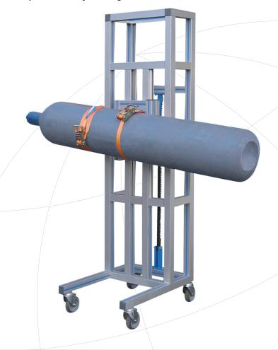
The cylinder can be rotated 360° continuously and locked at a position of 180° in lifted state. The unit is made of corrosion-free aluminium and can be xed to the oor by four screws. The cylinder tilting unit FSV-A facilitate the emptying of the cylinder after nished water pressure test according to the regulations for pressure tanks.
