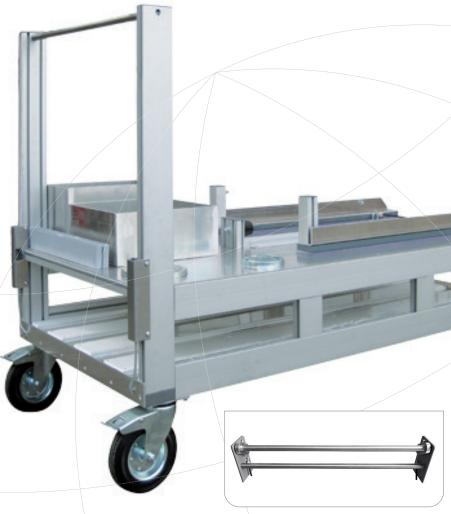
The wheels have Aluminium rims and solid rubber tyres to ensure the trolley has minimal rolling resistance and is easy to manoeuvre despite its weight even on rough ground. The single wheel load is 400 kg. The lower compartment of the trolley can be used to stored 4 Type A suction hoses; in the upper section the trolley has space for the storage of petrol canisters, ropes, Type B hose, fi re hydrant keys, 2 connector keys, as well as one Y-piece and one strainer
