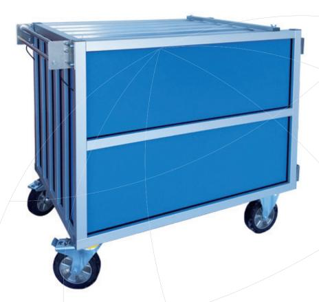
The trolley is fitted with two steering/ braking wheels and two fixed wheels and 5 hose storage compartments. The wheels have Aluminium rims and solid rubber tyres to ensure the trolley has minimal rolling resistance and is easy to manoeuvre despite its weight even on rough ground. The single wheel load is 400 kg.
